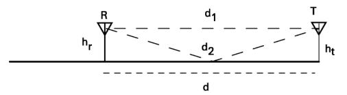
The setup is diagrammed above. The ISM transmitter (at 915 MHz) is placed on a metal cart on the sidewalk outside of the second floor of the EME building, across the bridge. You move along the sidewalk with the ISM receiver measuring field strength every 5 feet out to 270 feet. Keep the receiver at the same known height for all measurements.
